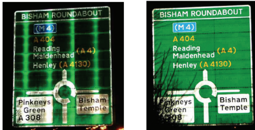
The same sign viewed at night, in the presence (left) and absence (right) of dew formation
