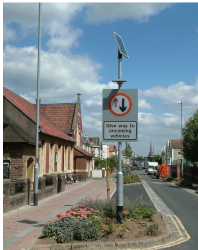
A traffic sign with solar powered lighting (photo courtesy of Solagen Ltd)
