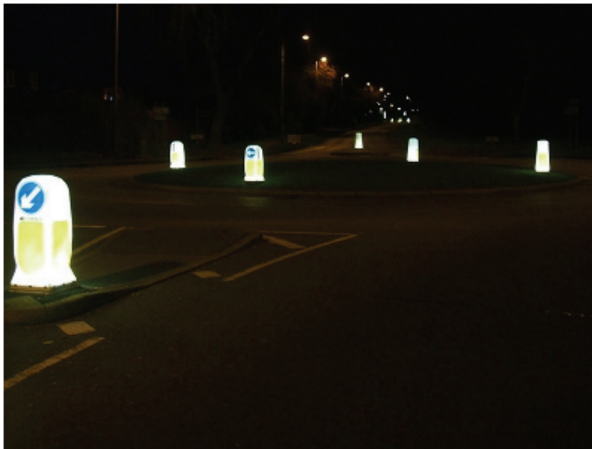
Figure 17 – Lit bollards can be seen clearly from any angle and at long distances (note the lights on the road in the far background of this picture are from distant bollards)
