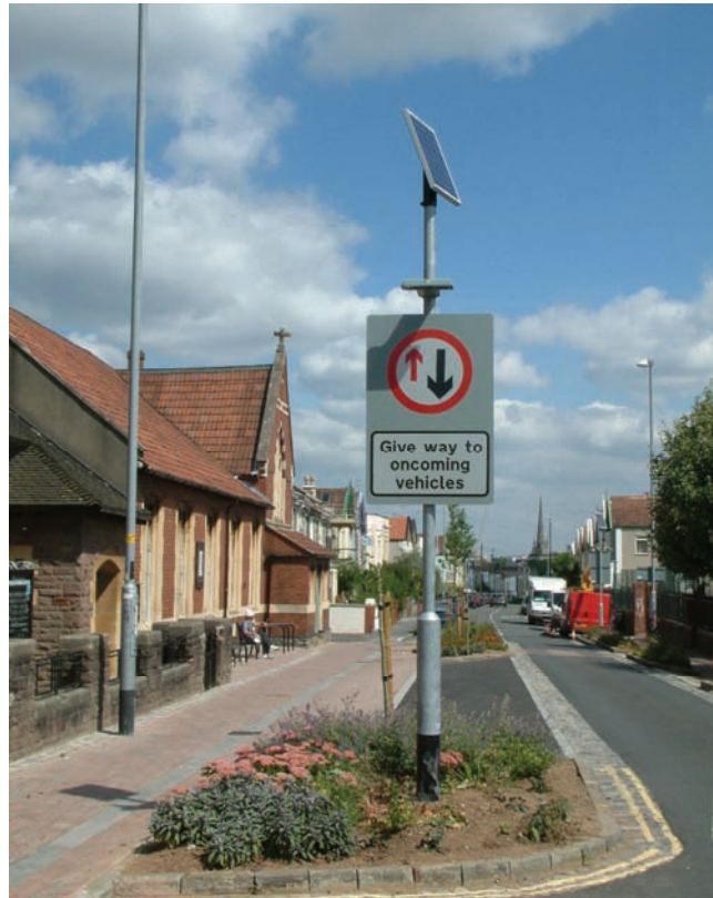
Figure 13 – A traffic sign with solar powered lighting (courtesy of Solagen Ltd)
